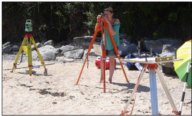
Intertidal surveying using a plane table, dumpy level and total station.
